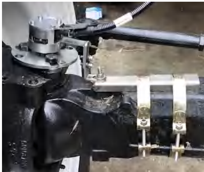
Figure 2.11 Installation example of angle sensor
