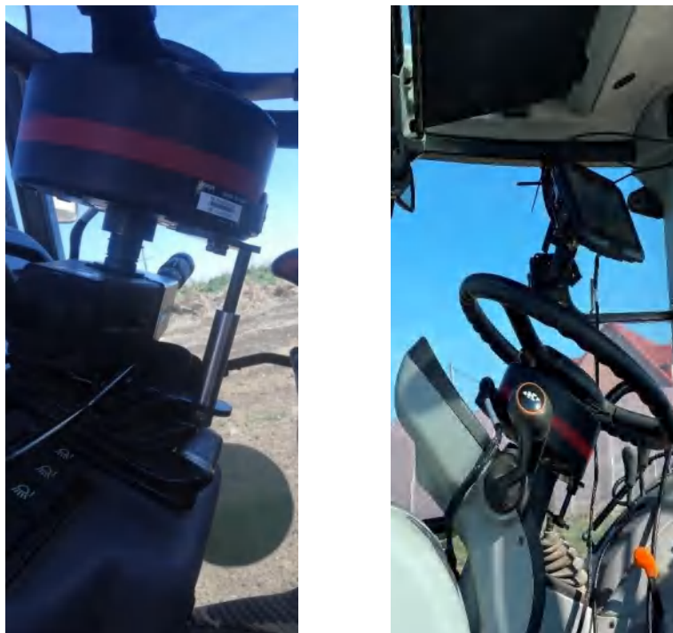
Figure 2.5 Installation example of bracket for fixating EMS2 Motor Wheel
