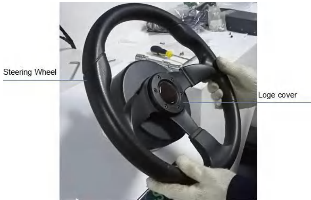
Figure 2.6 Installation example of EMS2 Motor Wheel
